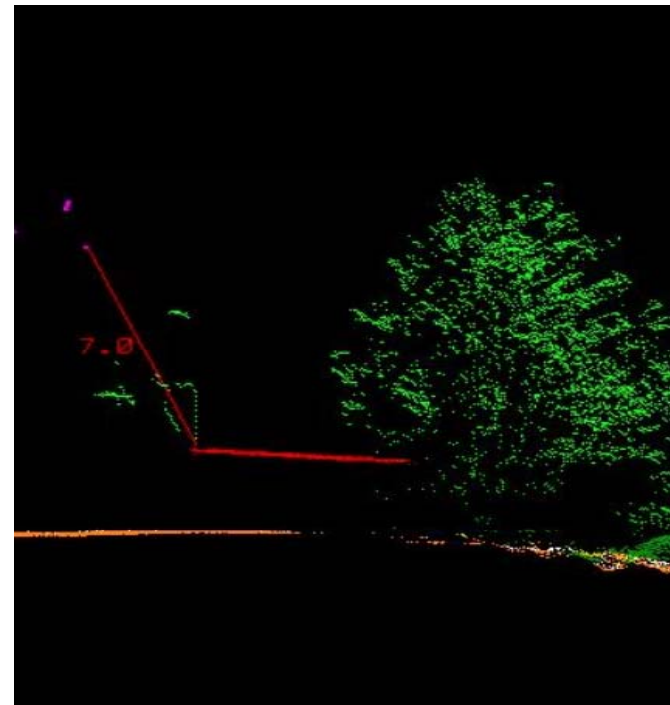
Signalling of critical situation measuring the real distance between conductors and objects
