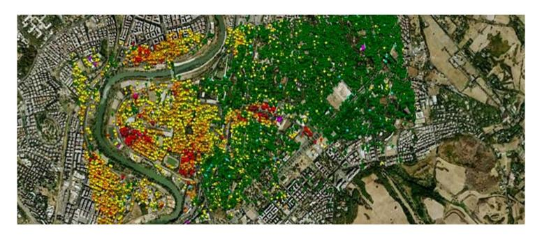
The project carried out for the Italian Space Agency was the result of an interesting research activity resulting in the development of software able to detect and measure with extreme precision the slow movements both of the ground and the buildings and infrastructures, through the analysis of COSMO-SkyMed Radar satellite data. The application, called SLIDE is the important result of the many years of experience gained by our team in SAR satellite data processing.
